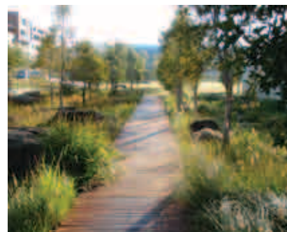
- Example of boardwalk through rain garden (Victoria Park, Zetland)
